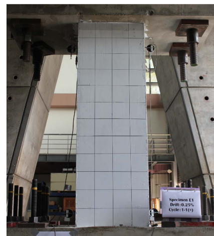
Fig. 2. (a) Multiaxial testing system (MATS); and (b) photograph of the test setup.
